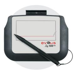
**Sig100 LITE** is a cost-effective signature pad, without LCD. Instead of the LCD screen, the pad is composed by a special hard-wearing writing surface for precise signature capture. Signature appears in real-time on the computer monitor, but not on the pad. It is the ideal product for applications where customers only need to provide a signature.
